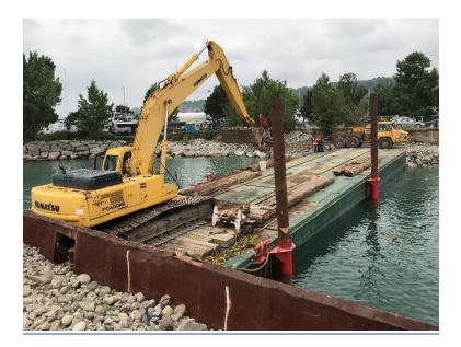
Construction: Steel Transport: Truckable Length: 40' or 20' Breadth: 10' Depth: 7' Gross weight: 35,700 lbs or 18,550 lbs Unloaded Displacement: 12" Available with a wide range of accessories
