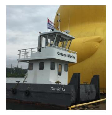
Construction: Steel Transport: Truckable Length: 7.77 m Breadth: 4.26 m Depth: 1.82 m Horsepower: 620 Propulsion: Twin Screw
